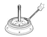
(Always allow your Rotovac to run for 10 minutes after installing new felt seals and before beginning to clean).
