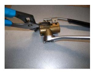
2. To remove the piston, first depress the trigger lever, then use your finger or a screw driver to push it through from the top of the valve.
