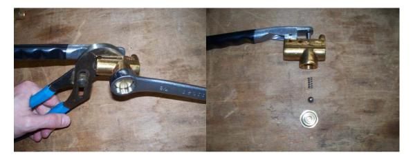
2. To remove the piston and plastic spacer washer, first depress the trigger lever, then use some needle nose pliers to remove the piston from the bottom of the valve.
