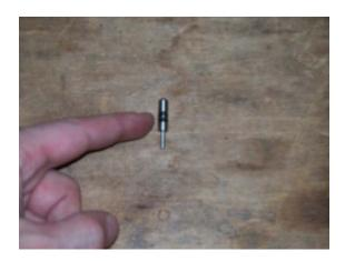
4. Use a liberal amount of Vaseline to lube the piston o-rings, then fully reinstall the piston. Install the metal washer before installing the plastic spacer washer.
