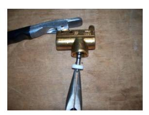
3. If needed, remove the two small o-rings from the piston and install new ones.
