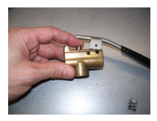
3. If needed, remove the two small o-rings from the piston and install the new ones.
