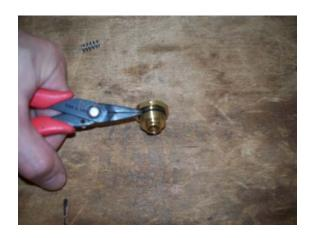
6. Place the spring inside the freeze plug and balance the ball bearing on top of the spring, then install the freeze plug using a 3/4" wrench.
