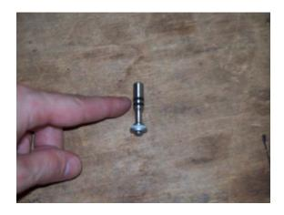
4. Use a liberal amount of Vaseline to lube the piston o-rings, then re-install the piston.
