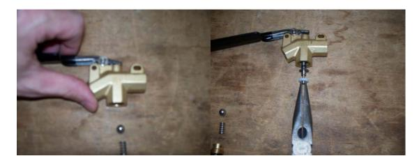
3. If needed, remove the two small o-rings from the piston and install new ones.
