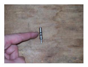
4. Use a liberal amount of Vaseline to lube the piston o-rings, then fully reinstall the piston and the plastic spacer washer.
