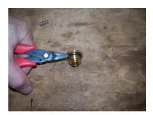
6. Place the spring inside the freeze plug and balance the ball bearing on top of the spring, then install the freeze plug using a 7/8" wrench.
