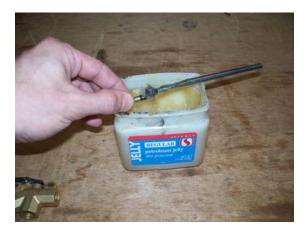
5. Remove the o-ring from the freeze plug and install the new o-ring.
