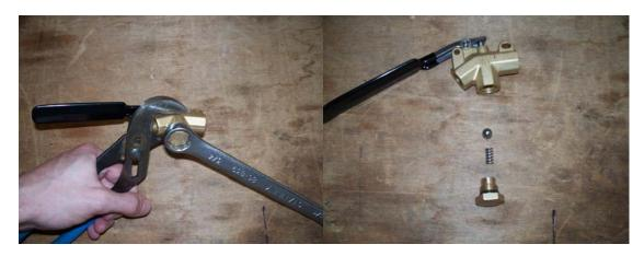
2. To remove the piston, first depress the trigger lever, then use some needle nose pliers to remove the piston from the bottom of the valve. The plastic spacer washer and metal washer will be on the piston.
