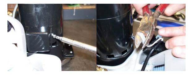
5) Using a pair of wire cutters, reach underneath the gearbox and cut the zip tie that fastens the vacuum hose to the vacuum chamber, then remove the vacuum hose.
