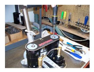
2) Remove the rotary union P/N:B-1763A from the right motor gearbox using 7/8" and ½" wrenches.
