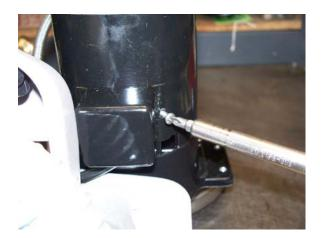
4) Fasten motor wiring to frame of Rotovac using two small zip ties.
