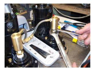
7) Use a Phillips screwdriver to install the top plate screws P/N: S-043 and the top plate P/N: F-043.
