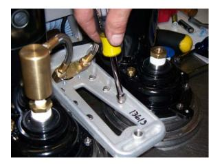
6) Wrap the threaded end of rotary union P/N: B-1763A with Teflon tape and use 7/8" and ½" wrenches to attach rotary union. Be sure to hand thread the rotary union on first to avoid cross-threading
