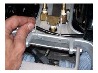
5) Use a 5/16" socket or nut driver to install the main frame screws P/N: S-040 to attach the right gearbox to the frame of Rotovac. Note: make sure to pull the right gearbox out as far as possible to the right to ensure proper leveling and even glide over carpet.
