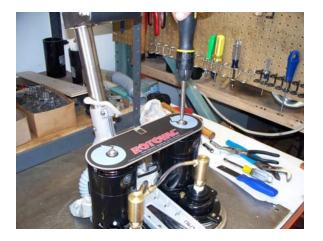
2) Remove the rotary union P/N: B-1763A from the left motor gearbox using 7/8" and  $\frac{1}{2}$ " wrenches.
