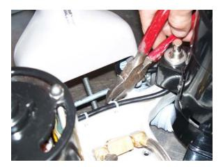
5) Make sure the machine is not plugged in and use a Phillips screwdriver to remove the wiring box on the <u>right</u> motor gearbox and use wire cutters to clip the two wire nuts, then remove the left gearbox wiring from the right switchbox.
