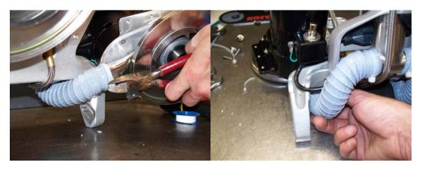
7) Unplug the cord located behind the vacuum hose at the base of the handle.
