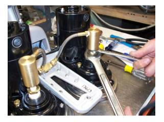
3) Use a 5/16" socket or nut driver to remove the three main frame screws P/N: S-040 from the left motor gearbox.
