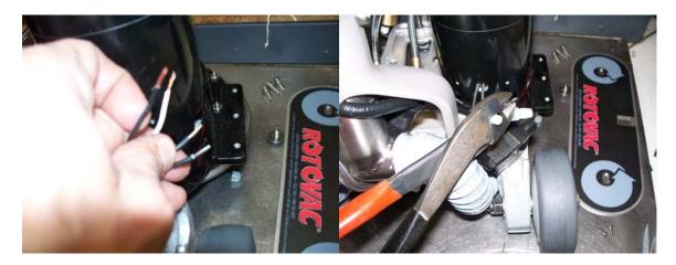
3) Use a Phillips screwdriver to attach the right switch box to the right gearbox.
