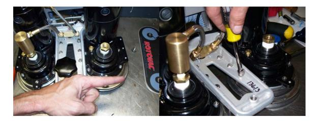
7) Wrap the threaded end of rotary union P/N: B-1763A with Teflon tape and use 7/8" and ½" wrenches to attach to the reducer bushing P/N: B-010. Note: Be sure to hand thread the rotary union the first few turns to avoid cross threading.
