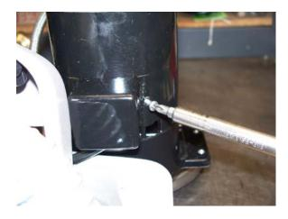
4) Fasten motor wiring to frame of Rotovac using two small zip ties.
