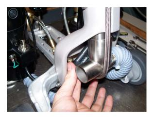
6) Use a 5/16" socket or nut driver to attach the main frame screws P/N: S-040, to the left gearbox to the frame of Rotovac. Note: make sure to pull the left gearbox out as far as possible to the left to ensure proper leveling and even glide over carpet.
