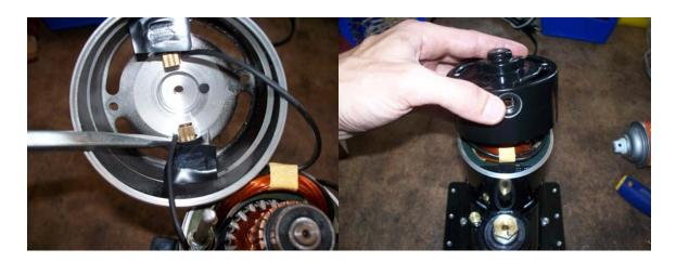
14) Use a 3/8" wrench or nut driver to install the acorn cap nuts P/N: S-048, being sure to tighten each side with equal force to ensure a balanced rotation of the armature.
