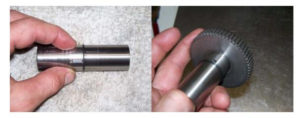
2) Place Female Shaft on end so that Large Gear is on top, and slide the Upper Gearbox Housing P/N: D2324 down onto it until firmly in place, being careful that the spring in the Drive Shaft Seal P/N S-028, does not fall out as the shaft is pushed through.
