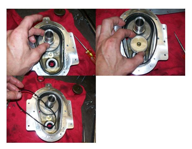
4) Slide Bottom Plate P/N: D-2319 onto Female Shaft. Note: It may be necessary to grease the inside of the large bearing and work the Bottom plate back and forth to walk it down the shaft. \*\*IMPORTANT – BEFORE BOTTOM PLATE IS SEALED DOUBLE CHECK THAT THE O-RING OIL SEAL HAS NOT MOVED OUT OF PLACE, AS THIS MAY CAUSE OIL LEAKS WHEN REPAIR IS COMPLETE.\*\*
