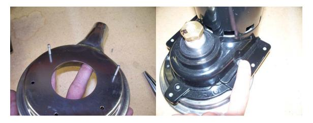
8) Fill the gearbox with 65cc's of 90 weight synthetic gear oil and use 7/16" wrench to install oil plug P/N: B-009. Check the oil level with a tooth pick and there should be a ½" of oil at the deepest point.
