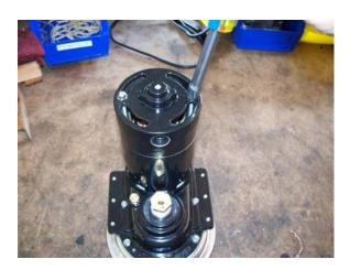
15) Use a flat head screwdriver to install Carbon Brushes P/N: C-018 and Carbon Brush Caps P/N: C-020. Note: Be sure that the curvature of the carbon brushes matches the rotation of the armature, or premature wear of the carbon brushes may occur.
