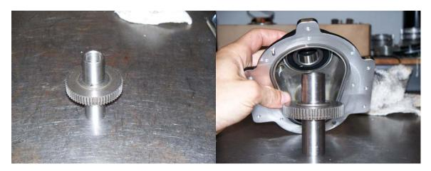
3) Place Upper Gearbox Housing upside down and install Gearbox Spacer P/N: D-2322 (on female shaft), Intermediate Gear P/N: B-2314 (onto large dowel pin in center of gearbox), and O-Ring Oil Seal P/N: O-111 (in groove around outside of housing). Note: Be sure that the rubber O-Ring stays in it's channel during the assembly process.
