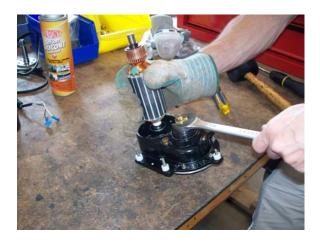
11) Install all-thread motor screws P/N: A-006 three or four turns.
