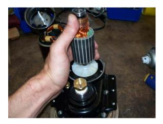
10) Wrap Reducer Bushing P/N: B-010 with Teflon Tape and hand tighten into female shaft. Wearing a heavy glove, grasp Armature firmly and use 7/8" wrench to fully tighten Reducer Bushing.
