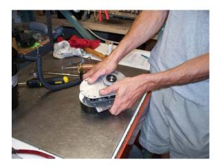
5) Use Phillips Screwdriver to fasten bottom plate screws P/N S-053 to bottom plate.
