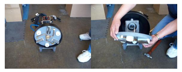
2) Locate and remove the five thumb screws on top of shroud and remove the grab handle.
