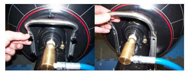
3) Remove shroud by gently freeing it from the shroud screws, tilting at a 45 degree angle and lifting upwards.
