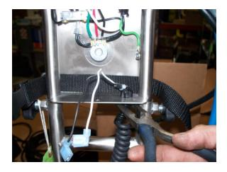
4) Use needle nose pliers to fasten White motor wire to post A+, and Black motor wire to post A-.
