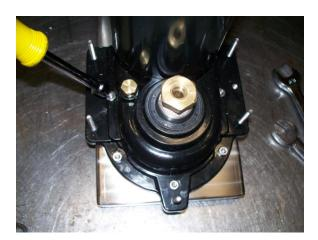
3) Run motor wire leads thru bottom of control box and use needle nose pliers to compress and re-secure strain relief.
