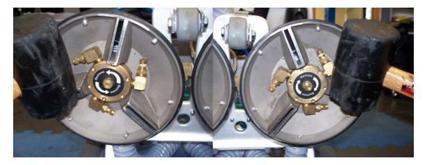
4) Should initial procedure prove unsuccessful it may be necessary to place 7/8" wrench onto reducer bushing and hold firmly while repeating step 3. Note: This method is mainly effective on the left side only. The reducer bushing on the right motor gearbox may unscrew if not secured tight enough.
