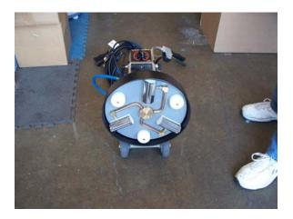
2) While facing the cleaning head, use your hand or foot to gently strike a shoe on the right side of the head downwards so that the head rotates clockwise until free from motor. If the head is stuck try a rubber mallet and a block of wood.
