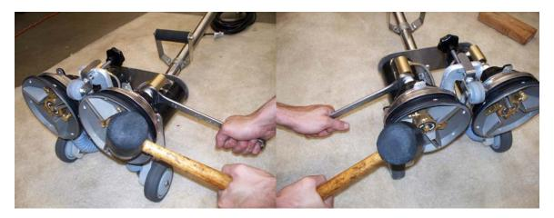
**\*\*** IMPORTANT – USE ONLY THE MINIMUM AMOUNT OF FORCE TO REMOVE CLEANING HEAD, AS REPEATED FORCFUL STRIKES MAY RESULT IN DAMAGE TO INTERNAL COMPONENTS **\*\***
