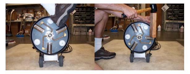
Head Stuck on 360 Removal Technique
