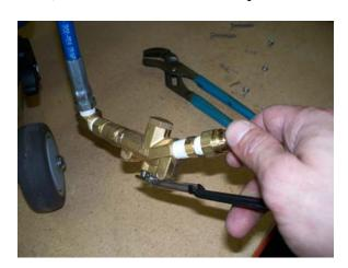
4) Place the two handle halves around the valve assembly so that the screw holes line up and use a Phillips screwdriver to install the five small handle screws.
