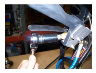
2) Use a 9/16" or crescent wrench to remove the hex nut P/N: V-053. Note: The hex nut may sometimes still be attached to the male quick connect.
