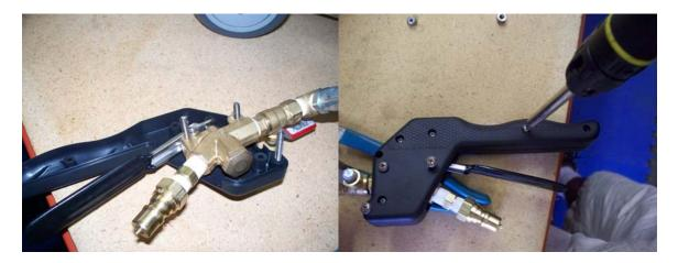
5) Hold handle assembly up to frame of machine and thread thru the 3 large handle screws, then use a Phillips screwdriver and a 3/8" wrench or nut driver to fasten handle to the frame. Note: Do not over tighten, as this could cause the handle to crack or break.
