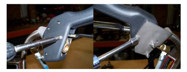
6) Use a ¾" deep socket or wrench to tighten the male quick connect. The hex nut will tighten at the same time as the male quick connect.
