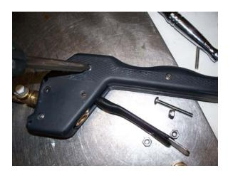
5) Grasp the valve assembly firmly with a pair of channel lock pliers and use a 9/16" or crescent wrench to remove the shut off valve from the main valve assembly.
