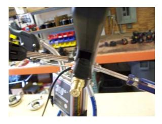
4) Use a Phillips Screwdriver to remove the five handle screws P/N: RV-544 and remove outer housing.
