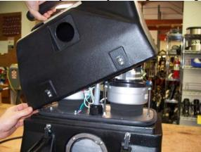
7) Cut the zip ties holding the wiring in place and unplug the red float switch wires.
