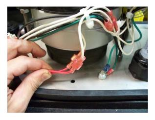
8) Place the deck plate assembly on its side and remove the float switch shroud.
