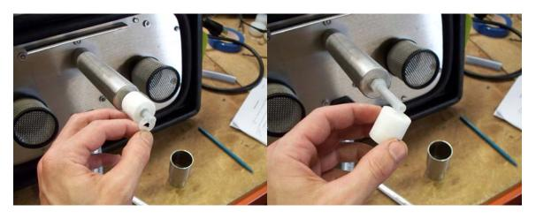
10) Use a <sup>1</sup>/<sub>2</sub>" wrench to unscrew the level switch, and pull the wires through the float switch tube.
