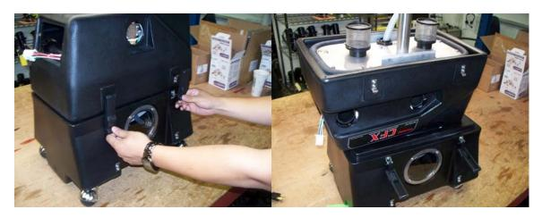
4) Use a 5/16" wrench or nut driver to remove the eight deck plate screws
