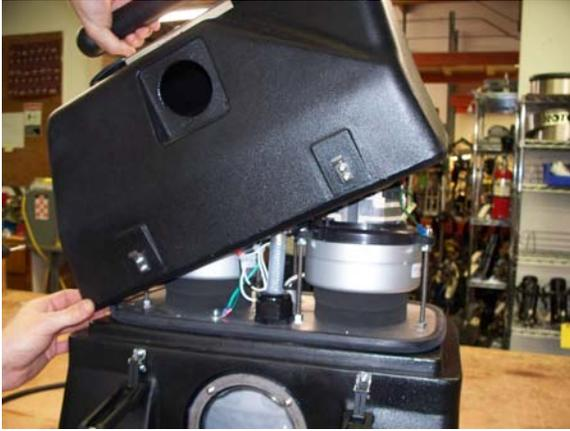
7) Use a pair of needle nose pliers to unplug the wires from the pump to the wire bundle.
