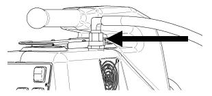
Secure the discharge end to sink or toilet making sure it will not fall out and flood the area with dirty water. **SUPER IMPORTANT:** Make sure to **secure your clear empty hose** into a toilet or drain so that it will not accidentally fall out.
