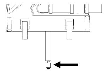
Make sure the empty pump screen filter on the end of the hose is resting on the very bottom of the recovery tank (shown below)
