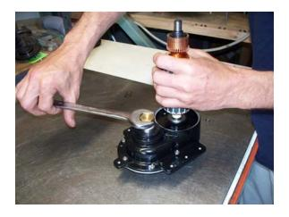
6) Remove the Armature. Note: If Armature is stuck, it may be necessary to grasp the armature firmly in one hand and strike the upper gearbox with a rubber mallet, alternating between the front and back of the gearbox until the armature comes free. The armature base bearing may be still attached to the armature upon removal.
