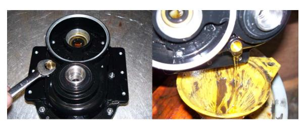
8) Use Phillips Screwdriver to remove the three bottom plate screws P/N: S-053 and remove bottom plate P/N: D-2319. Note: If bottom plate is stuck it may be necessary to use a flat head screwdriver to pry open the gearbox, being careful not to damage the gearbox housing. In some cases a press or vice may be required.
