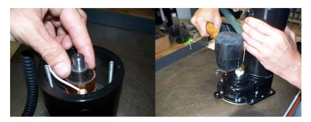
4) Remove all-thread motor screws P/N: RV-434.
