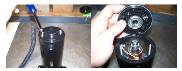
3) Remove Motor Tube P/N: RP-201(kit). Note: If Motor Tube is stuck, grasp the tube tightly and gently strike the gearbox on top of the reducer bushing with a rubber mallet. \*\* IMPORTANT – DO NOT STRIKE OR JAR THE MOTOR TUBE, AS THIS MAY CAUSE FRACTURES TO THE MAGNANT WITHIN. \*\*
