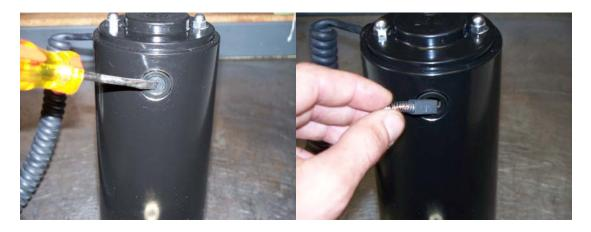
2) Use 3/8" Nut Driver to remove Acorn Nuts P/N: S-048 from Motor Cap. Remove motor cap P/N: RP-201(kit), shim washers P/N: RP-231, and spring washer P/N: RP-232 from top of armature.
