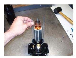
5) Grasp the Armature firmly in one hand and use a 7/8" wrench to loosen and remove the reducer bushing P/N: B-010.
