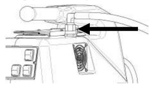
Secure the discharge end to sink or toilet making sure it will not fall out and flood the area with dirty water. **SUPER IMPORTANT:** Make sure to **secure your clear empty hose** into a toilet or drain so that it will not accidentally fall out.
