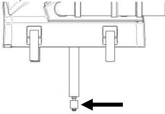
• Make sure the empty pump screen filter on the end of the hose is resting on the **very bottom** of the recovery tank (shown below)
