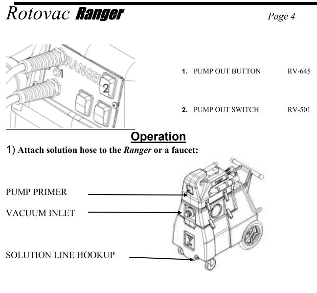
1. The Ranger fill hose can be attached any faucet that is higher that the fill port of the water tank. care should be taken to make sure that the fill hose is secure before turning on the water.
